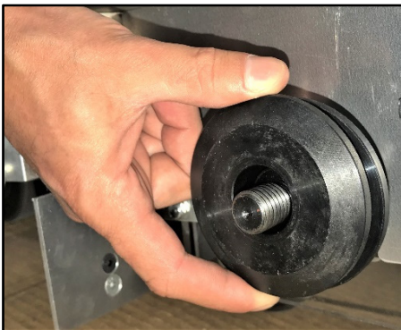
Removing the Outer Flange
