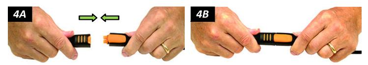
4) Connect the electrical connectors (figs. 4A-B and figs. 4C-D).
