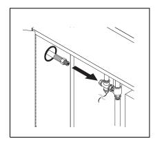
**STEP 3**: Connect high pressure hose from pressure washer when connecting to burner module outlet.
