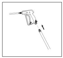
**STEP 4:** Attach high pressure wand to spray gun of connected pressure washer (Not Included).
