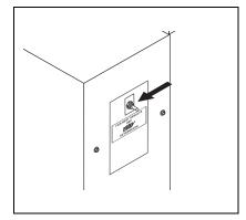
**STEP 6:** Turn on burner switch. Pilot ignition will begin to spark. Confirm pilot light ignition, if unsuccessful, turn off switch and turn on again. If pilot continues to spark, but not light, consult troubleshooting guide.
