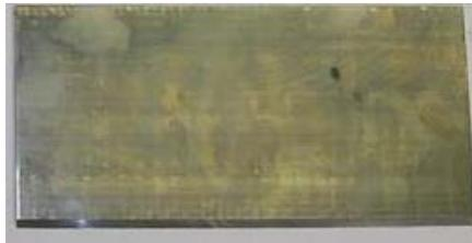
For carpet, rubberized and elastomeric coatings, a carpet blade should be utilized. The 90° wings on each end of the blade will help keep the removed material manageable. See figure 3.3.2.
