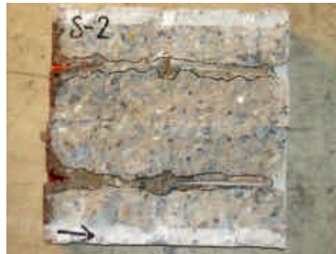
S-2 Neoprene Rubber Ring (LEAK)
