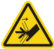
Pinch Point Hazard
