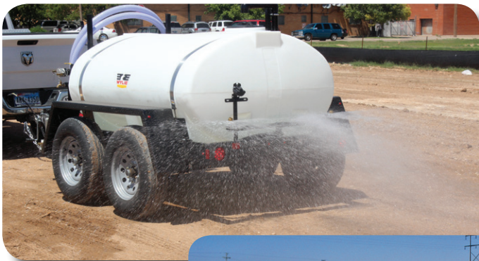
Spray Bar covers up to 25" with TeeJet brass nozzles.
