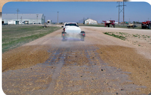
Spray Bar covers up to 25" with TeeJet brass nozzles.
