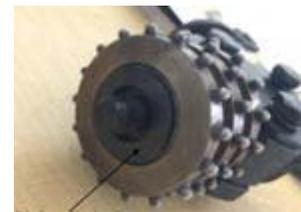
5. Slide Belleville washer onto shaft against the outer bearing cover.
