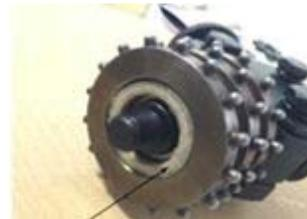
4. Slide outer bearing cover onto shaft against the felt washer.
