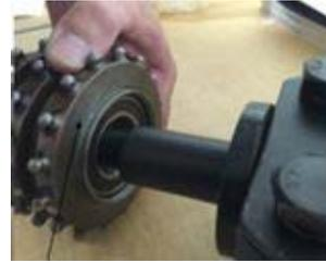
3. Slide felt washer onto the shaft into the space between the cutter edge and the bearing edge.
