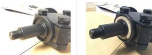
2. Slide cutter assembly onto shaft up to the backing plate.
