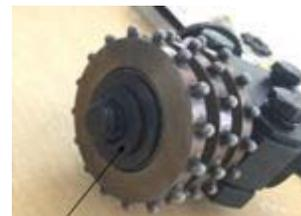
6. Place hex nut onto shaft. Tighten so the nut is tight but the cutters can freely rotate on their bearings (if no rotation, the nut is too tight).
