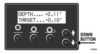
**Long Press:** Lowers the drum to Cut Depth Target.
