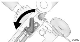
3. Depress Engine Kill Button and turn Engine Power Switch to "OFF".
