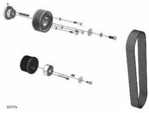
Remove belt guard, belt, and both pulleys from the flail (low speed) setup machine.
