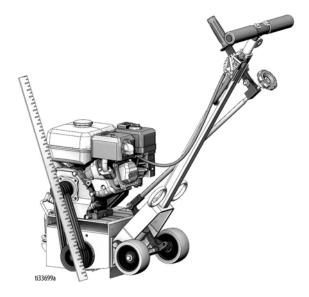
8. Verify pulleys are properly aligned, tighten everything down and re-check pulley alignment one last time.
