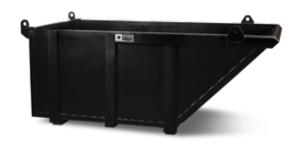
To dump the skip, the two forward slings are disconnected from the lifting eyes with the lifting line slack. The skip is then lifted with the rear slings still connected, effectively dumping the load from the sloped end.
