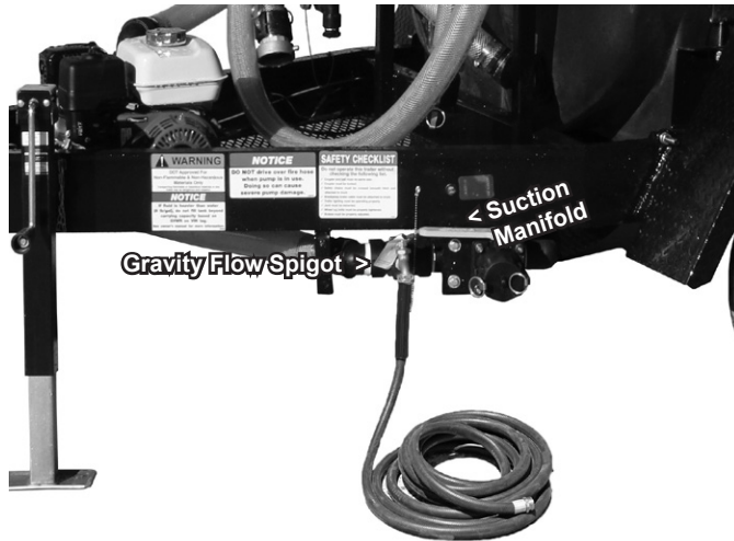
Figure B4 Water Wagon Plumbing
