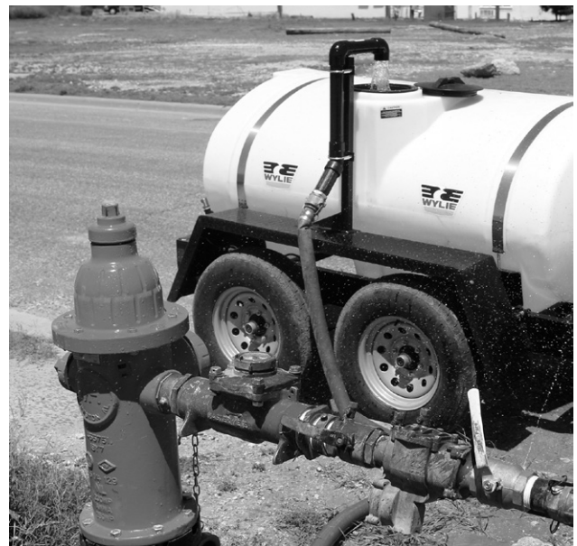
Figure B2 Filling Tank Through Anti-Siphon Fill
