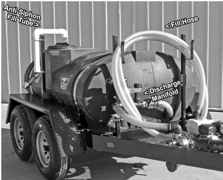
Figure B1 Water Wagon Plumbing
