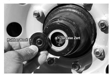
Figure B20 Accu-Lube Hub
