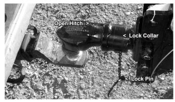
Figure C2 Hitch in Open Position
