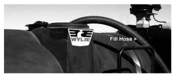
Figure C9 Filling Tank Through Fillwell
