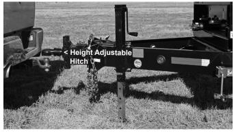
Figure C5 Adjust Hitch Height for Level Trailer
