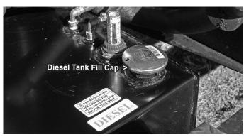
Figure C6 Diesel Tank Fill Cap
