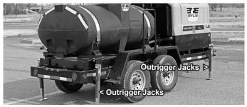
Figure A6 Set Outrigger Jacks to Stabilize Trailer
