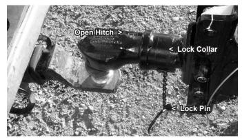
Figure B2 Hitch in Open Position
