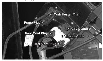
Figure A19 Heat Cord Connections
