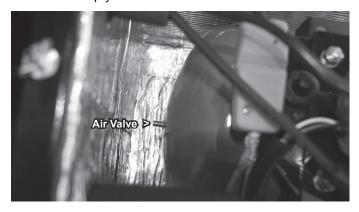
Figure C15 Pressure Tank Air Valve
