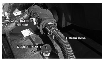
Figure A22 Draining Tank
