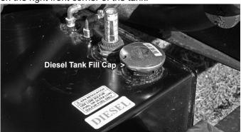
Figure A7 Diesel Tank Fill Cap
