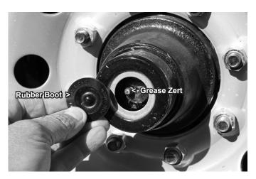
Figure A27 Accu-Lube Hub
