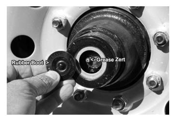
Figure C26 Accu-Lube Hub
