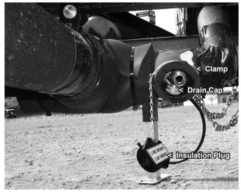
Figure B18 Suction Line Drain Cap
