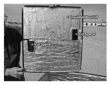
Figure B15 Lid with Spacers in Cold Weather Position; Rotate Spacers for Hot Weather
