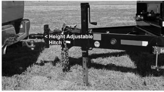
Figure B5 Adjust Hitch Height for Level Trailer
