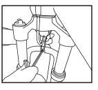
3) Place the front light, fender, before the front fork hole, and fasten this with the
