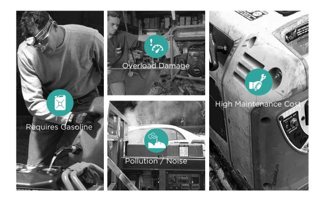
"Stale fuel is the No.1 cause of generator starting problems Manufacturers advise adding fuel stabilizer to the gas to minimize fuel breakdown, varnish and gum buildup."
