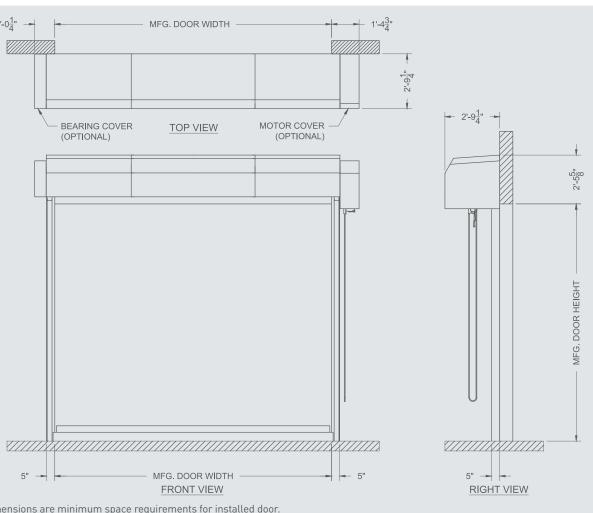
All indicated dimensions are minimum space requirements for installed door. Note: Based upon individual environmental safety considerations, extra safety components such as push buttons, detectors and covers may be required.
