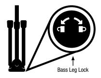
To open or close legs, turn base leg lock clockwise to the unlocked position. When in desired position, turn base leg lock counter clockwise to the locked position.
