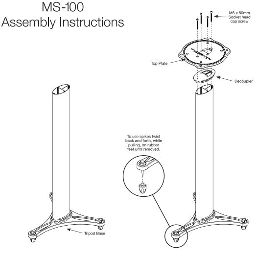
Users planning to add extra weight to their stand with sand or shot should do so prior to adding the second decoupler. We recommend using small bags to add the sand to avoid unwanted spillage. Add to the large channel of the stand. The two smaller channels are for cables and should remain open.
