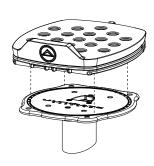
Place Adjustable platform onto top plate. Line up spiked feet with top plate grooves.
