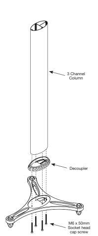
Place one of the decouplers on one of the ends of the column. Make sure the two large holes on the decoupler line up with the two channels of the column. The third channel should be covered. Line up screw holes on the decoupler with the tripod base and attach using four M6 x 50mm socket head cap screws.
