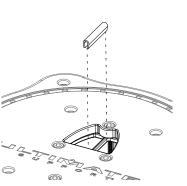
Place web cover over the wall separating the two channels.
