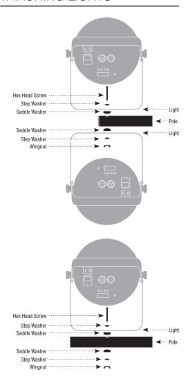
The Fly Point Mountable Lighting Bar includes its own hardware for mounting lights. Use the diagram above to attach the lights on either side of the speaker.
