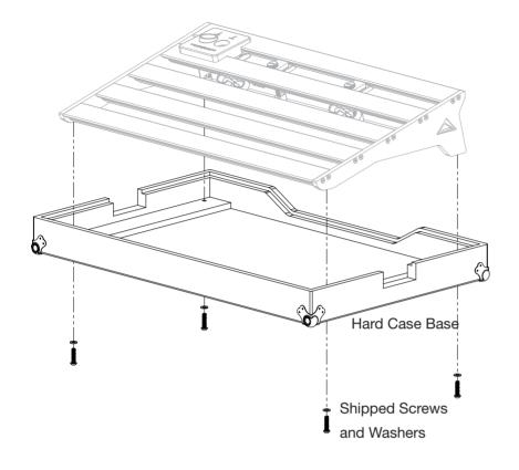
Open the hard case and place lid off to the side. Remove the four washers and screws from the base; freeing the pedalboard from the hard case base. Set aside the four washers and screws you have removed as you will use the packaged screws and feet instead.
