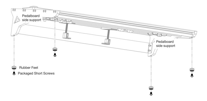
OPTIONAL: In case you would like to use the pedalboard by itself we have included an extra set of small pedalboard feet. Detach the pedalboard from the case. Locate the holes underneath the pedalboard side supports, then attach the four rubber feet using the packaged short screws.
