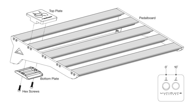
To attach mic adapter to pedalboard, place top plate in between any two rows. The logo will be at the bottom. Place second plate under pedalboard, lining up holes on both plates. Use the two hex screws to clamp plates together. To adjust the mic adapter, remove hex screws, place top plate at desired location and repeat the steps to attach the mic adapter.
