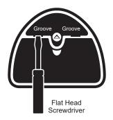
Using a flat head screwdriver, find the two grooves and pry top plate.
