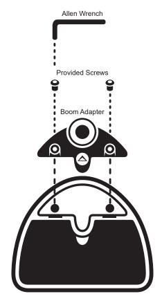
Place the boom adapter on the keyboard stand cap. Use the two provided screws and Allen wrench to attach the boom adapter.
