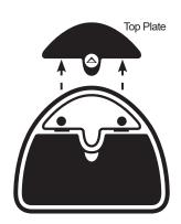
Remove the top plate off the keyboard stand cap.
