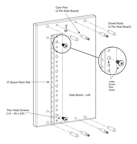
Screw cam pins into top and bottom of side board. Cam pins screw into inside holes. Next push the dowel rods into top and bottom of side board using the outside holes.
