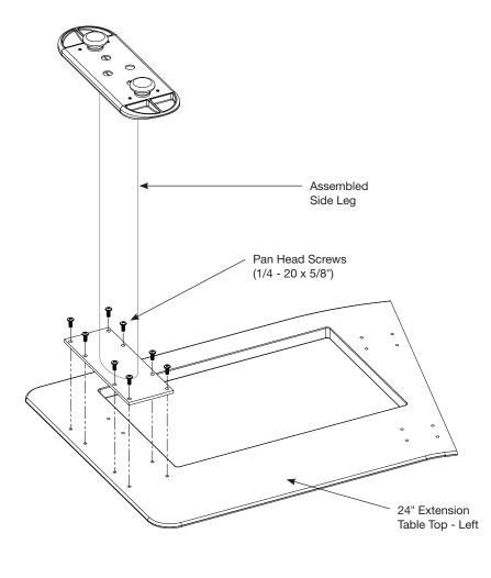
Lay 24" extension face down with holes facing up. Place assembled side leg on 24" extension and line-up all eight holes. Attached table top and side leg together with eight pan head screws  $(1/4 - 20 \times 5/8")$ .
