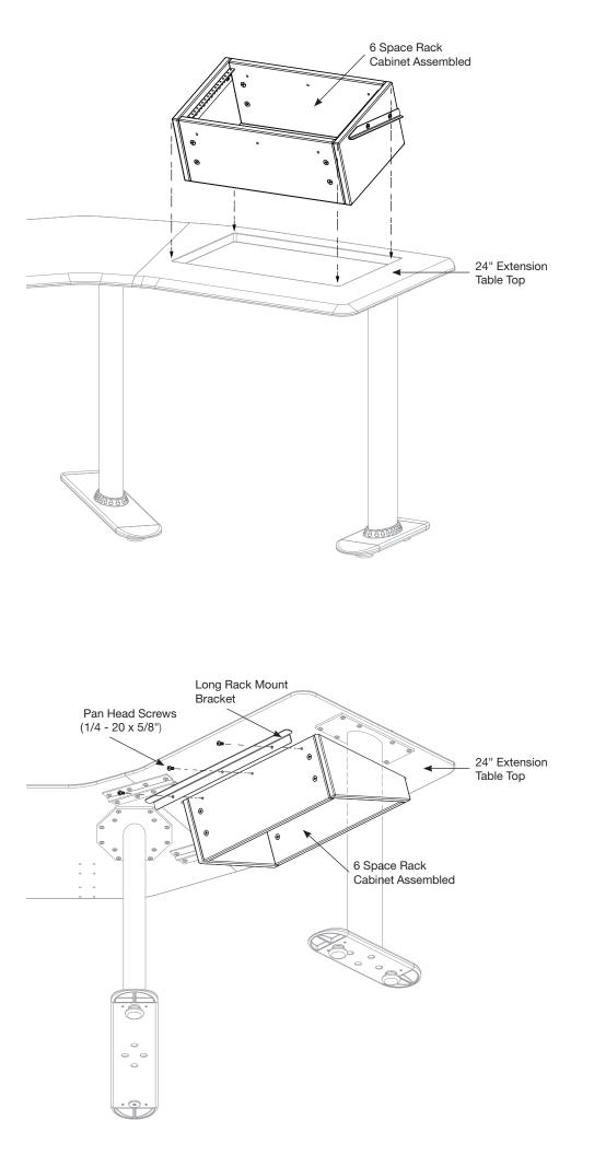
Place 6 space cabinet through opening on 24" extension. Rack mount brackets will rest on top of 24" extension table top.
