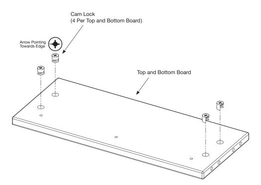
Lay Top and bottom board with large holes facing up. Push the four cam locks into large holes on the top and bottom board. The arrow on the cam locks should be pointing towards the edge.
