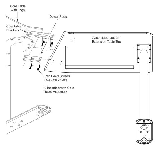
Slide the 24" extension onto the three dowel rods and line-up holes with the two brackets on the core table. Use the eight pan head screws (1/4 - 20 x 5/8") that came with the core table assembly (Box 1) to attach 24" extension.
