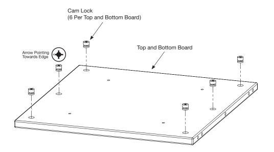
Lay Top and bottom board with large holes facing up. Push the six cam locks into large holes on the top and bottom board. The arrow on the cam locks should be pointing towards the edge.
