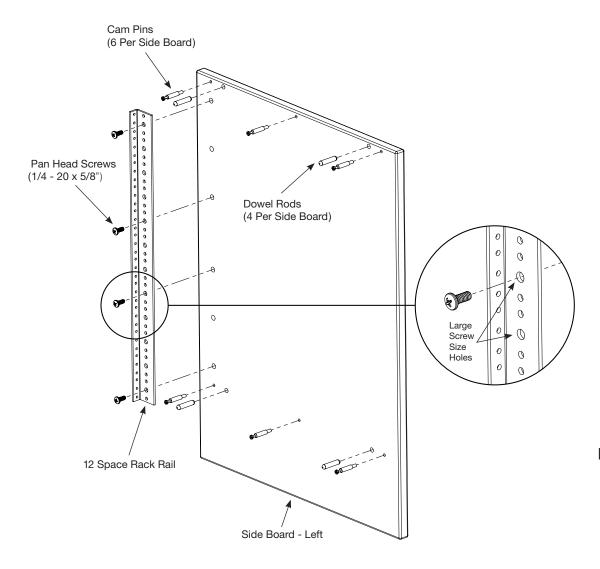
Screw cam pins into top and bottom of side board.
