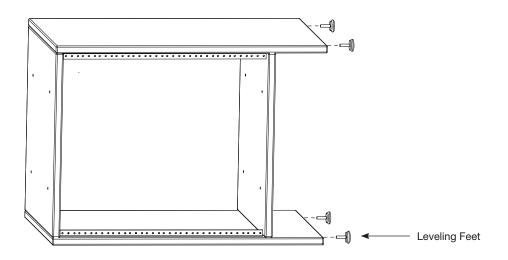
Attach leveling feet to assembled rack cabinet.
