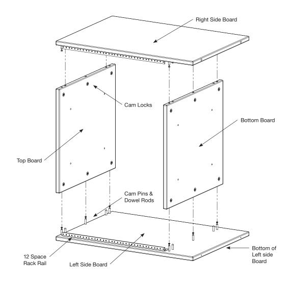
Lay the left side board down with the rack rail facing up. Slide the top and bottom board onto dowel rods and cam pins. On top and Bottom boards make sure the cam locks are facing the bottom of the left side board.
