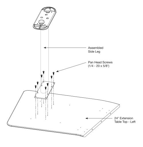
Lay 24" extension face down with holes facing up. Place assembled side leg on 24" extension and lineup all eight holes. Attached table top and side leg together with eight pan head screws (1/4 - 20 x 5/8").
