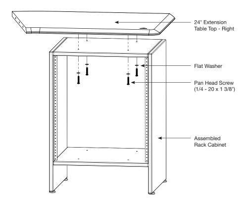
Stand rack cabinet up, place right 24" extension table top on rack cabinet and line-up holes. Attached table top and cabinet together with four pan head screws (1/4 - 20 x 1 3/8") and flat washers.
