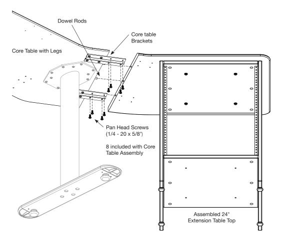
Slide the 24" extension onto the three dowel rods and line-up holes with the two brackets on the core table. Use the eight pan head screws (1/4 - 20 x 5/8") that came with the core table assembly (Box 1) to attach 24" extension.
