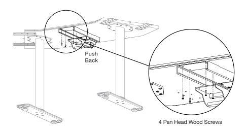
Push keyboard tray back to access the other four keyboard tray assembly holes in the front. Use four pan head wood screws to finish attaching keyboard tray assembly to core table. You may need to loosen back screws to line-up front screw holes, then tighten screws again.
