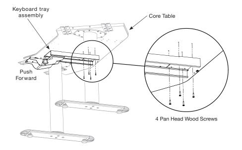
Pushed keyboard tray forward. Line-up the back four center holes of the core table with the back holes of the keyboard tray assembly.
