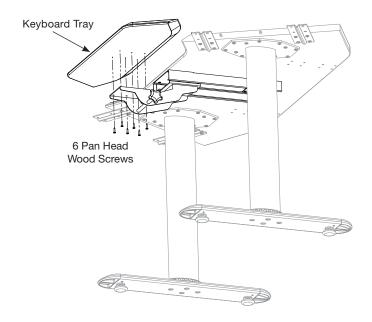
Push forward the keyboard tray assembly. Line-up holes on the keyboard tray assembly with keyboard tray. Use six pan head wood screws to attach.
