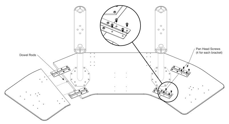
Attach left and right gussets to 12" extensions using the four pan head screws for each side. Make sure that gusset's holes line up with leg and 12" extension holes. Attach gussets to legs using the two self-drilling screws for each side.
