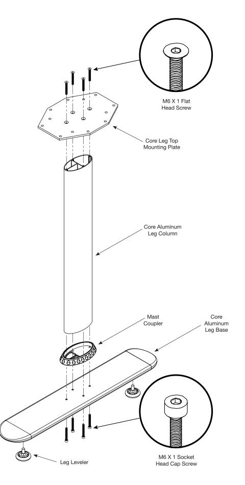
Place core leg top mounting plate on aluminum leg base, lining up the holes. Use the four flat head screws provided to attach plate to leg base. Use M4 hex wrench to tighten flat head screws.
