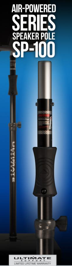
The new SP-100 speaker poles feature an expanding cylinder system that will firmly fit multiple speaker sockets from 1- 3/8" to 1-1/2" diameter. Using a 2mm hex wrench, the adapter can also be removed to provide standard M20 threading, allowing your SP-100 speaker pole to be a truly universal solution.
