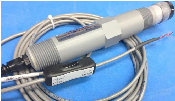
Figure 2 - 2017 version of R65 series ORP sensors with rocker switch for range selection
