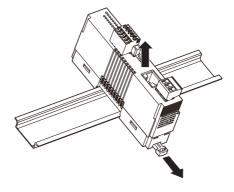
Note: When the unit is mounted on a DIN rail attached on the wall surface in vertical direction, use of an attachment plate to prevent the module from sliding down is recommended.
