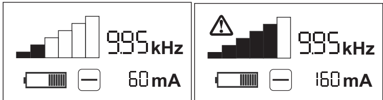
Fig. 7: Energizing for electromagnetic location – main view Left image: Signal strength in ES1 range (safe-to-touch range) Right image: Signal strength in ES2 range ( Notice symbol)
