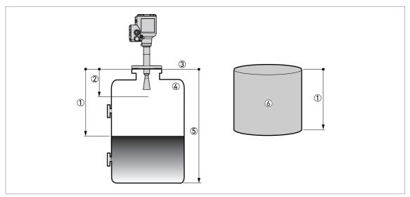
Figure 10-4: Measurement definitions: distance
