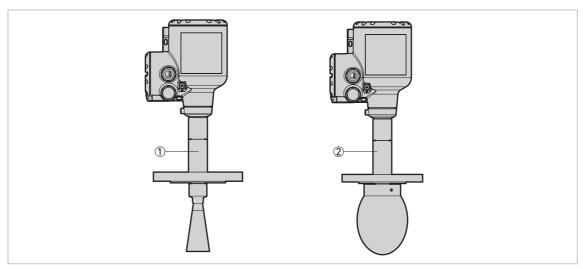
Figure 2-2: Types of antenna
