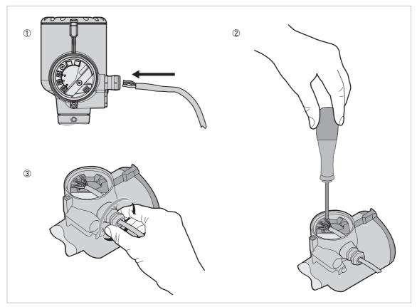
Figure 4-3: Procedure for electrical installation
