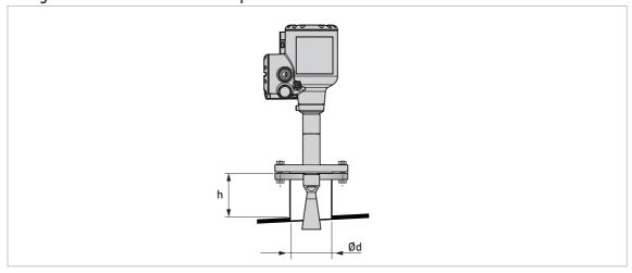
Figure 3-10: Flange connections: installation procedure
