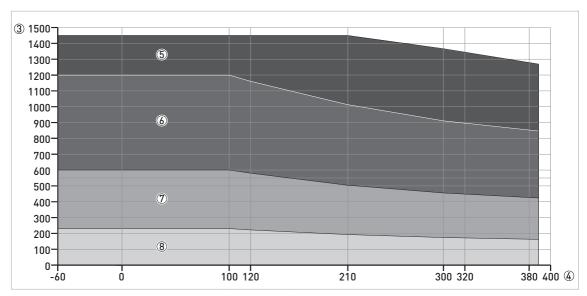
Figure 8-9: Pressure / temperature de-rating (ASME B16.5), flange and threaded connections, in  $^\circ F$  and psig
