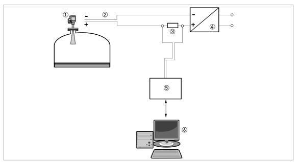
Figure 4-8: Point-to-point connection (non-Ex)
