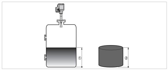
Figure 10-5: Measurement definitions: level
