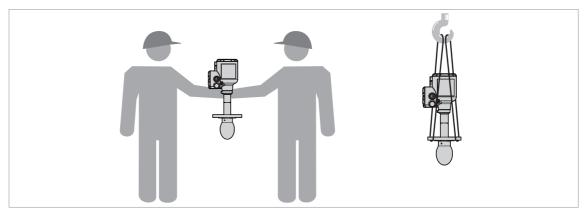
Figure 3-2: How to lift the device
