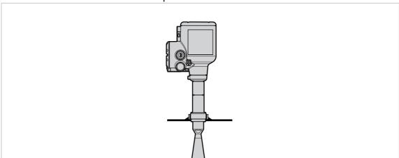
Figure 3-12: Threaded connections: installation procedure
