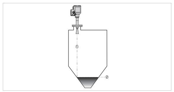
Figure 3-7: Tanks with dish-shaped or conical bottoms
