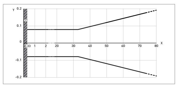
Figure 8-3: Measuring accuracy (graph of measuring accuracy in inches against measuring distance in ft)
