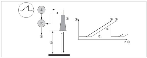
Figure 8-1: Measuring principle of FMCW radar
