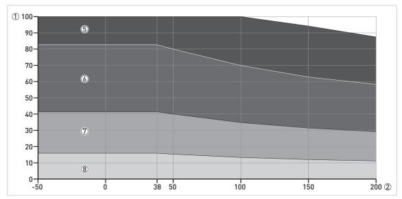
Figure 8-8: Pressure / temperature de-rating (ASME B16.5), flange and threaded connections, in  $^{\circ}$ C and barg
