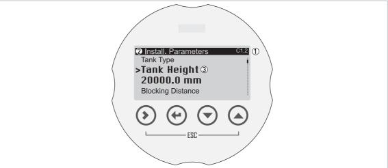
Figure 5-2: Display screen layout in Program mode
