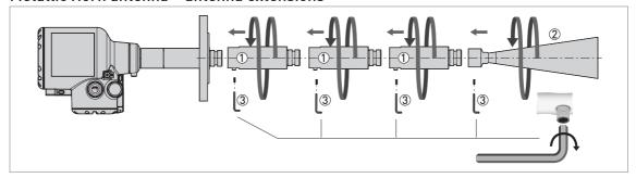
Figure 3-20: Metallic Horn antenna – how to attach antenna extensions
