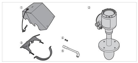
Figure 3-24: Equipment needed to assemble the weather protection
