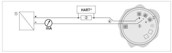
Figure 4-6: Electrical connections for non-Ex devices
