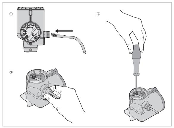
Figure 4-3: Procedure for electrical installation
