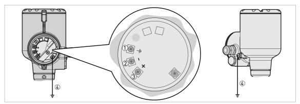
Figure 4-1: Terminals for electrical installation: standard cable gland
