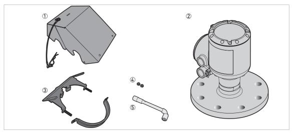
Figure 3-16: Equipment needed to assemble the weather protection
