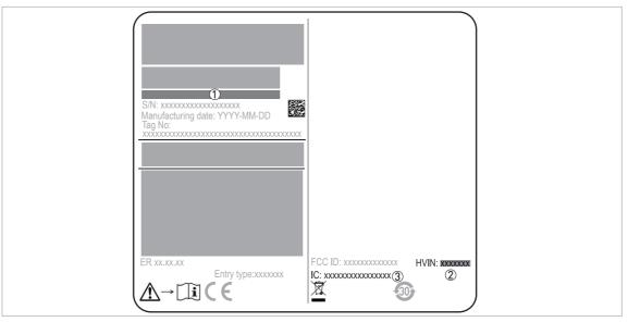
Figure 1-3: Canada: radio approval information on the nameplate
