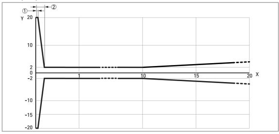
Figure 8-2: DN40 (1 $\frac{1}{2}$ ") Lens antenna: measuring accuracy (graph of measuring accuracy in mm against measuring distance in m)
