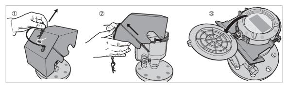
Figure 3-18: How to open the weather protection
