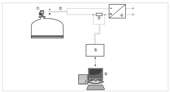
Figure 4-8: Point-to-point connection (non-Ex)
