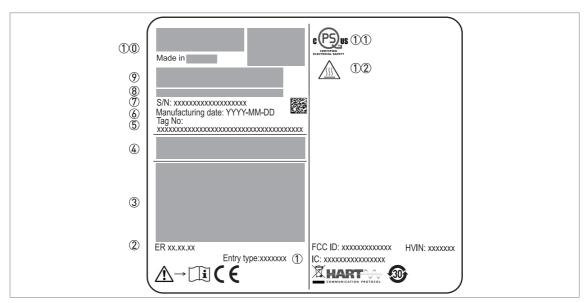
Figure 2-5: Non-Ex nameplate attached to the housing
