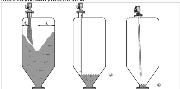
Figure 3-4: Recommended nozzle position for solids
