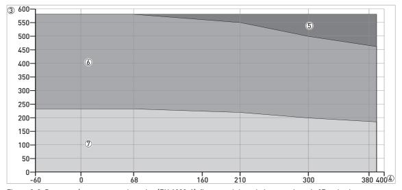
Figure 8-9: Pressure / temperature de-rating (EN 1092-1), flange and threaded connections, in  $^\circ F$  and psig
