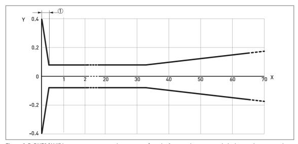
Figure 8-5: DN70 (1½") Lens antenna: measuring accuracy (graph of measuring accuracy in inches against measuring distance in ft)
