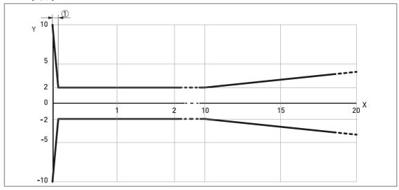
Figure 8-4: DN70 (23/4") Lens antenna: measuring accuracy (graph of measuring accuracy in mm against measuring distance in m)
