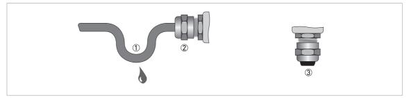
Figure 4-7: How to make the installation agree with protection category IP68
