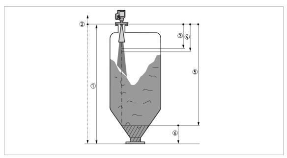
Figure 6-7: Distance measurement
