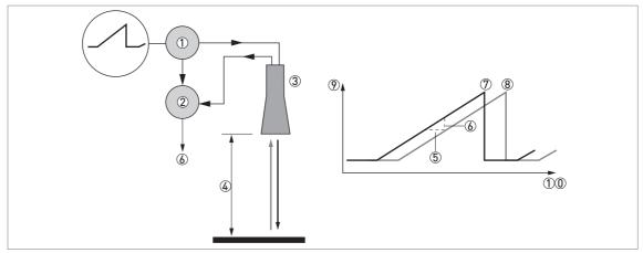
Figure 8-1: Measuring principle of FMCW radar
