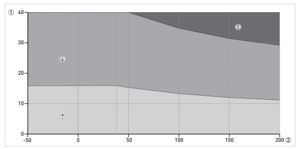
Figure 8-10: Pressure / temperature de-rating (ASME B16.5), flange and threaded connections, in  $^{\circ}$ C and barg
