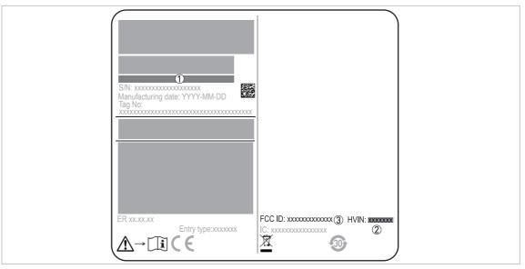
Figure 1-2: U.S.A.: radio approval information on the nameplate
