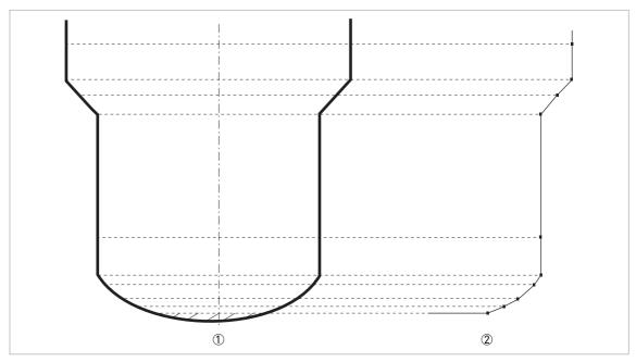
Figure 6-9: A plot of points for a volume or mass table
