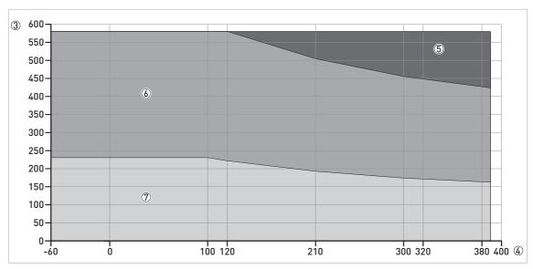
Figure 8-11: Pressure / temperature de-rating (ASME B16.5), flange and threaded connections, in  $^\circ F$  and psig
