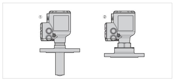
Figure 2-2: Types of antenna
