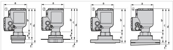
Figure 8-13: DN70 /  $2\frac{3}{4}$ " Lens antenna versions
