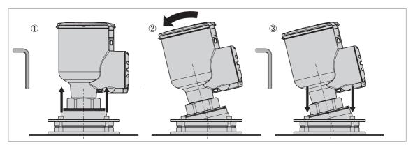
Figure 3-13: How to tilt the device
