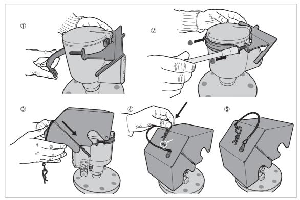
Figure 3-17: Installation of the weather protection
