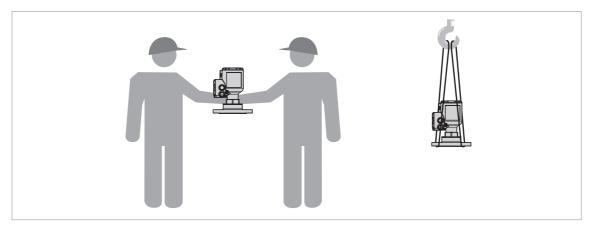
Figure 3-2: How to lift the device
