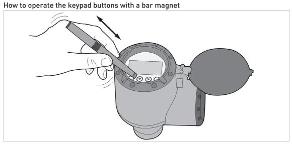
Figure 5-4: How to operate the keypad buttons with a bar magnet
