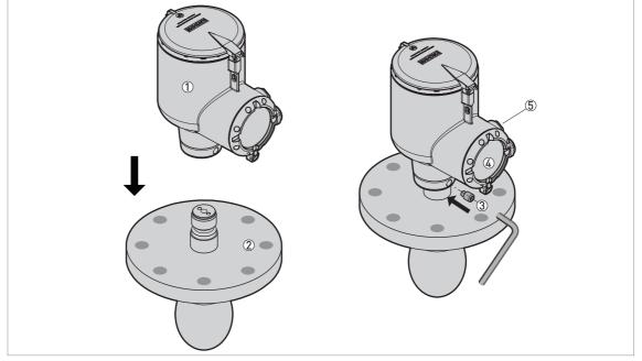
Figure 7-3: Procedure 3: How to attach the REFLEX RC Series signal converter
