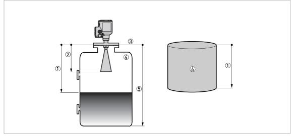
Figure 10-4: Measurement definitions: distance
