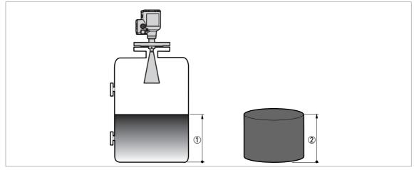
Figure 10-5: Measurement definitions: level
