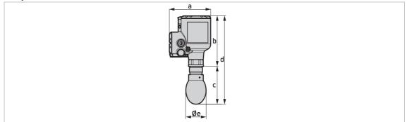
Figure 8-13: Drop antennas with threaded connections
