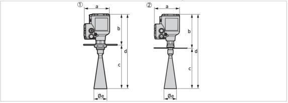
Figure 8-12: Metallic Horn antennas with low-pressure flange connections
