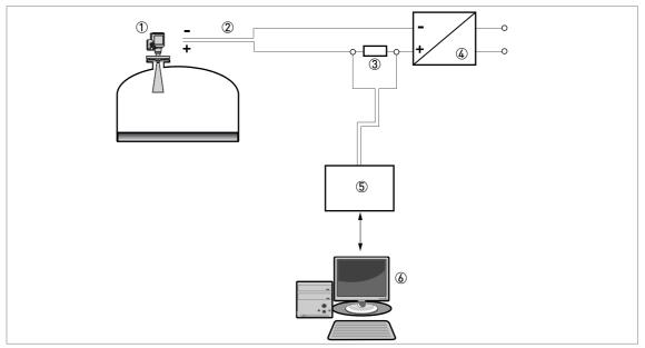
Figure 4-8: Point-to-point connection (non-Ex)
