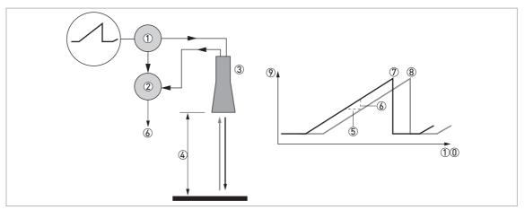
Figure 8-1: Measuring principle of FMCW radar
