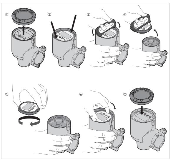
Figure 3-19: How to turn or remove the display module (option)
