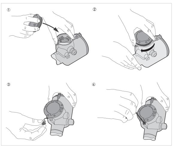
Figure 4-4: How to close the terminal compartment cover
