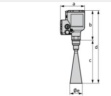
Figure 8-10: Metallic Horn antennas with G or NPT threaded connections
