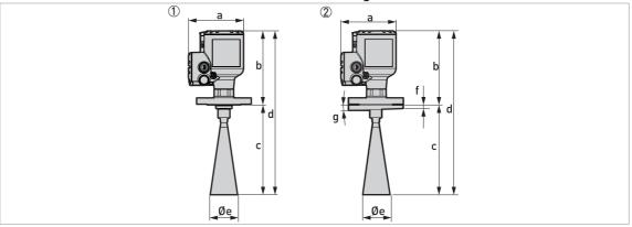
Figure 8-11: Metallic Horn antennas with standard flange connections
