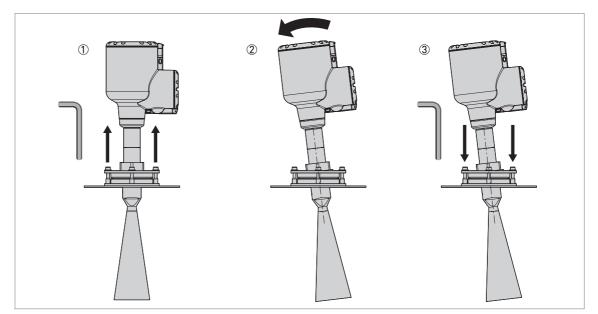
Figure 3-18: How to tilt the device
