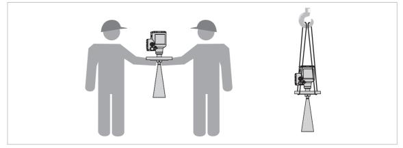
Figure 3-2: How to lift the device
