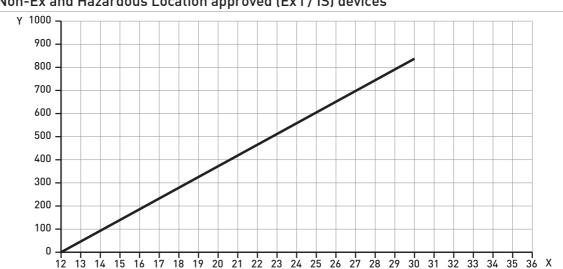
Use these graphs to find the minimum power supply voltage for a given current output load.
