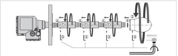
Figure 3-15: Drop antenna – how to attach antenna extensions
