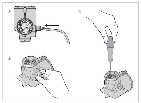
Figure 4-3: Procedure for electrical installation
