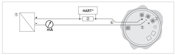
Figure 4-6: Electrical connections for non-Ex devices
