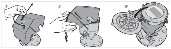
Figure 3-22: How to open the weather protection
