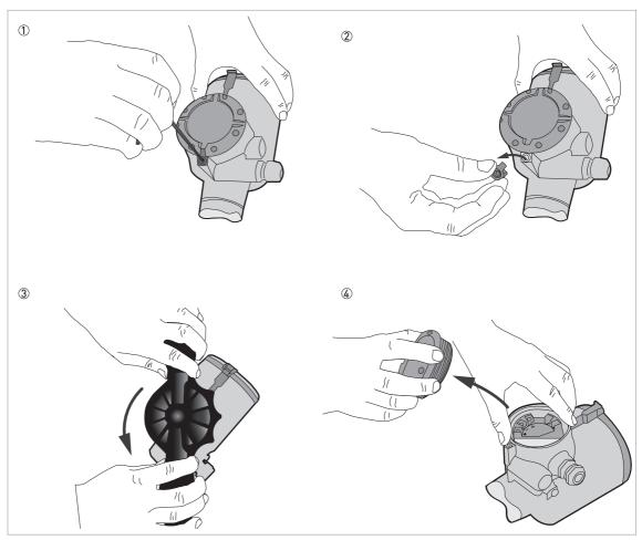
Figure 4-2: How to open the terminal compartment cover
