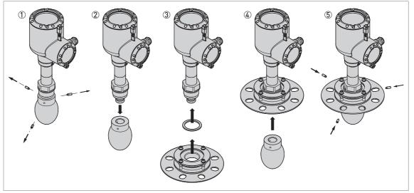
Figure 3-17: Device with a Drop antenna
