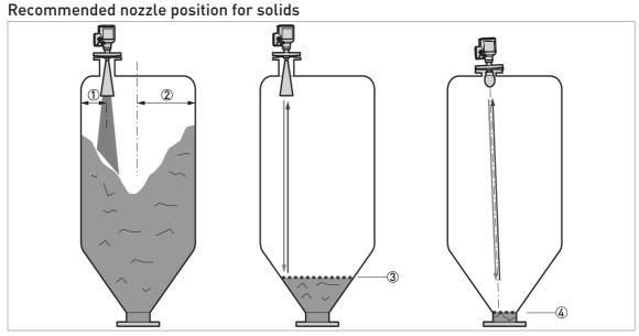
Figure 3-4: Recommended nozzle position for solids
