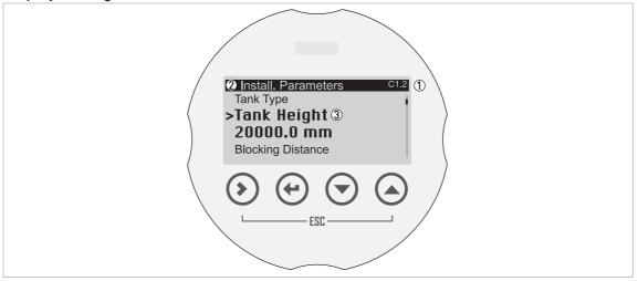
Figure 5-2: Display screen layout in Program mode
