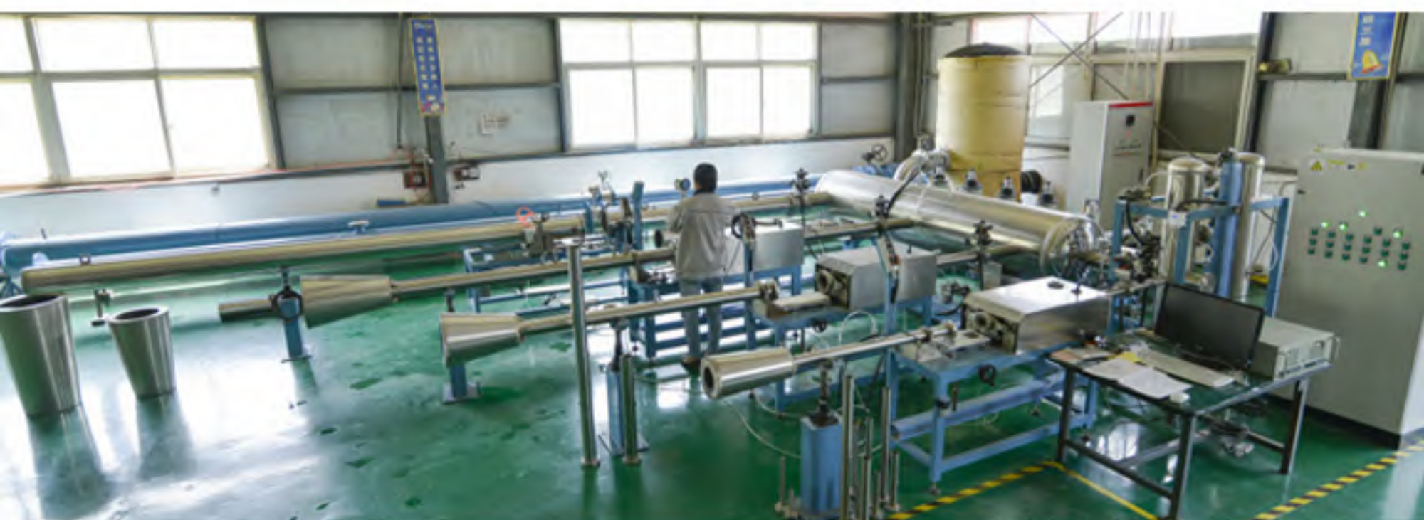
Critical Flow Nozzle Calibration Device DN15-DN200
