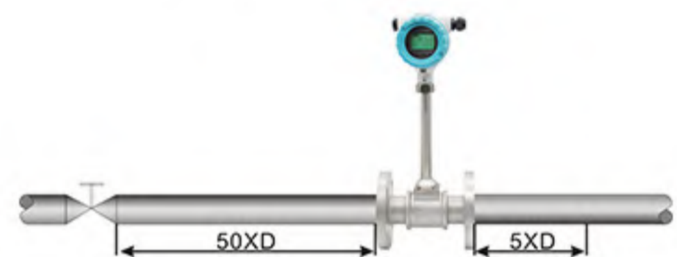
Regulating Valve, Half-open Gate Valve
