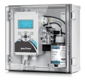
PACON 4900 is a compact, easy to operate and accurate on-line analyser from JENSPRIMA for the automatic on-line measurement of phenolphthalein alkalinity and quality control of boiler water. The titrimetric colour change principle allows the measurement of high and low ranges by selecting different reagents. Low maintenance and low reagent consumption for long continuous operation. Standard 4-20mA and RS485 Modbus outputs for easy integration into your existing control system.
