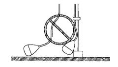
6.3.2 Keep a certain free surface area to operate without interference. Locate away from the tank wall.
