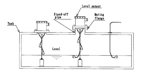
Keep an ample space for maintenance and inspection. Make sure the sensor is installed in an area which meets the following conditions.
