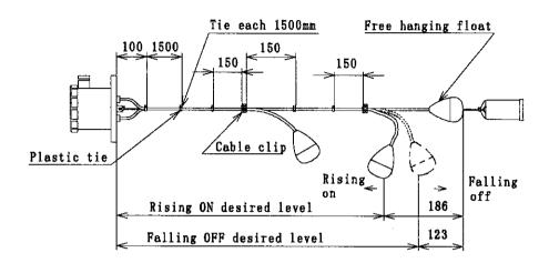
(6) Cut the useless part of cable and connect lead wires to the terminals. In case of triple level detection, wire 21, 2 and 23 are as shown on the right.
