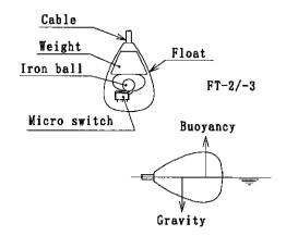
the microswitch opening and closing. Principle of operation for the FT55/77 is same, but those floats are non-submersible designs at SG=1.0.
