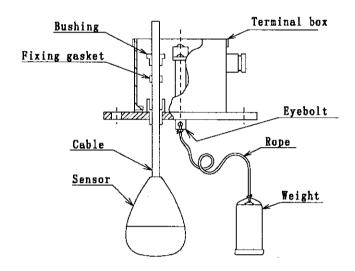
(3) Set the float on the rope according to specified measuring length with the cable clip. See page 9.
