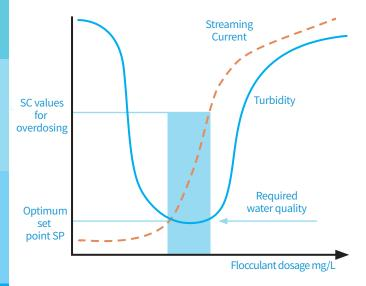
The streaming current is used to continuously measure the electric charge on the tiny suspended particles and colloids in the liquid. The electric charge is measured by electronic signal processing.
