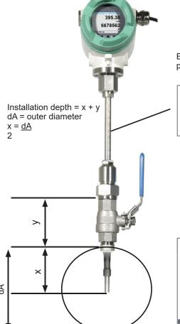
Engraved depth scale for precise installation
