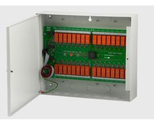
The 32 way relay panel accepts relay data from the combi control unit. It must have a unique address between 128 and 255. This can be selected using the SW1 binary address switch (see example). Ensure that its address does not conflict with another CAN bus device.
