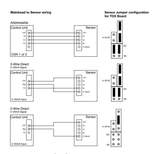
Controller to sensor wiring
