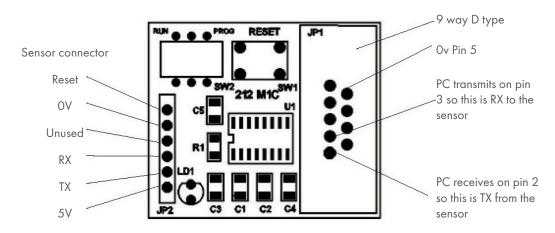
When programming the sensor processor, the Run and Prog slide switch SW2 is set to Prog but under normal circumstances, this switch should be in the Run position.
