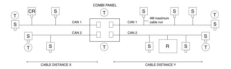
Maximum cable distance for CAN signal X+Y = 1 km
