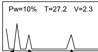
#2: read obstacle's secondary echo
