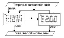
Pressing **[UP]** key or **[DOWN]** key in this screen will cycle the display between E2.00, E0.00 above.
