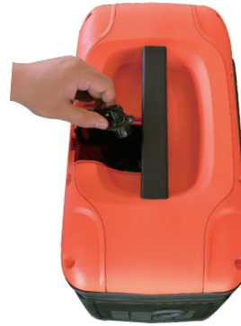
Figure 2 - Removing the spark plug cover
