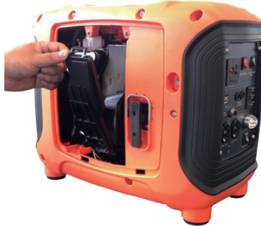
Figure 6 - Removing the air filter cover
