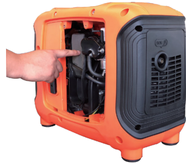
Figure 7 - Removing the air filter
