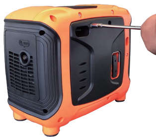
Figure 1 - Removing the Maintenance Cover Plate
