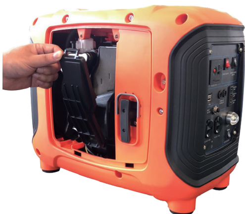
Figure 4 - Removing the air filter cover
