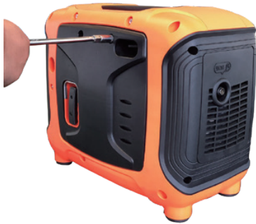
Figure 5 - Removing the Maintenance Cover Plate
