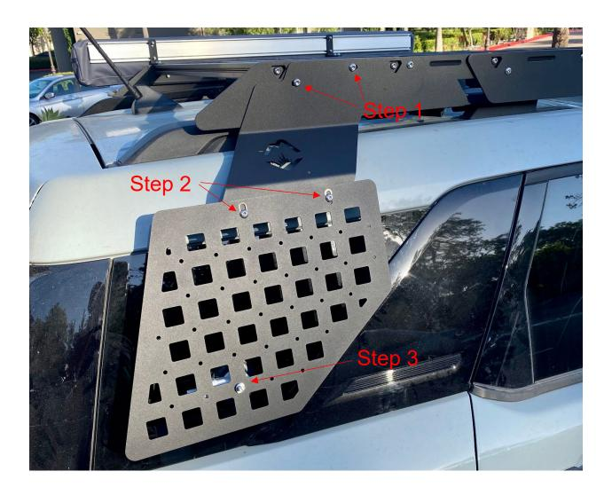
Step 1 – Fasten the mounting bracket to the rear side panel of the rack
