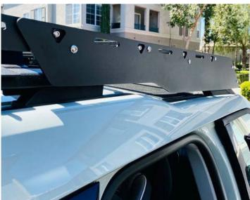
Make sure the side panels align with the contour of the car!
