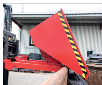
Emptied by activating release point 1
