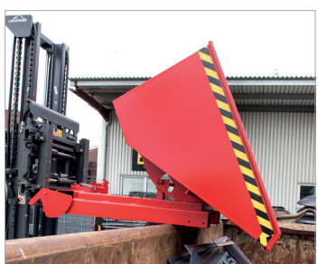
Emptied by activating release point 2
