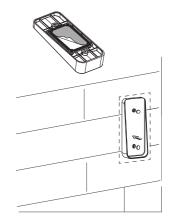
(3) Remove the battery door cover and insert two AAA batteries. Replace the battery cover.
