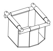
Place the rope through the holes in the wooden rods, then make triple knots beneath the rod.
