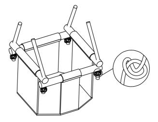
Hang the swing to the swing frame. Before using, add weight to the seat and do practice swings to ensure the knots and other pieces are fixed properly.
