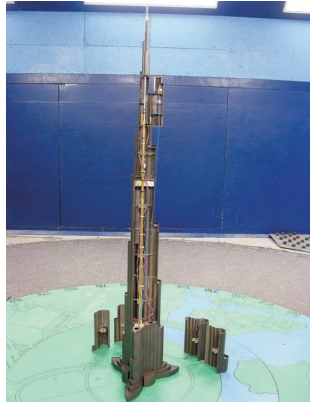
▲ Figure 3.8: Example of aeroelastic model illustrating inner spine for providing stiffness scaling, and segmented outer shell to provide shape and mass scaling. © RWDI
