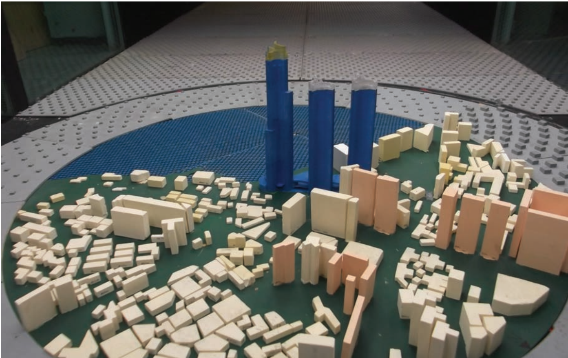
▲ Figure 3.2: Haeundae Beach Towers, Busan, Korea. Wind tunnel testing performed in February 2012. © BMT Fluid Mechanics
