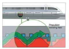
fig 4. Section showing propulsion system for typical mag lev train. Source: Maglev train elevation. [Online Image] Available: http://www.transrapid.de/cgi-tdb/en/basics.pr q?session=d82f8833463f50c9&a\_no=41,
